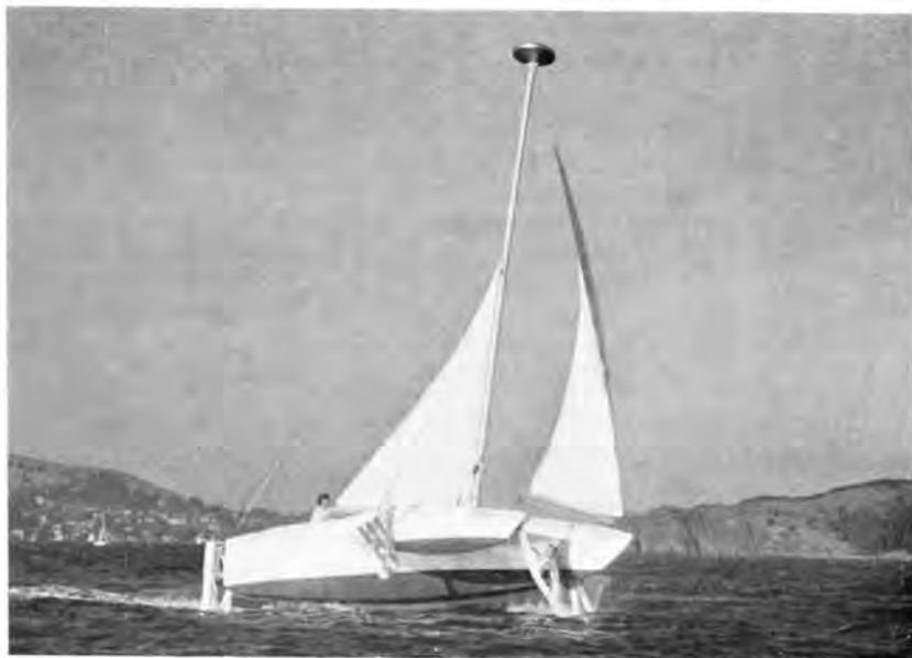
WILLIWAW at speed. Note weather foil is out of the water
