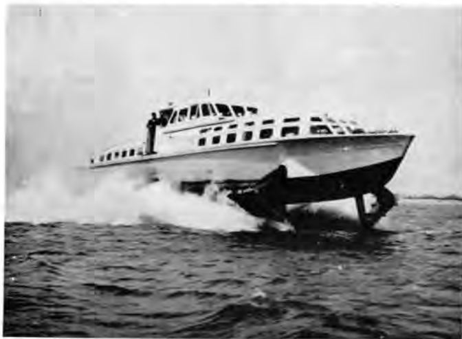
Fig. 6 Von Schertel 27 ton Passenger Ferry foil-borne Speed about 40 knots
