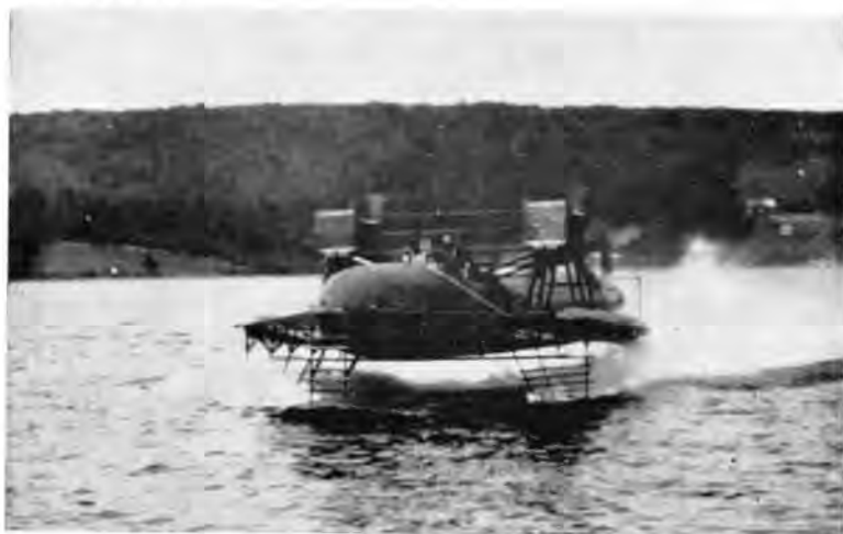
Fig. 5 The Bell HD4 1918. Speed 60 knots
