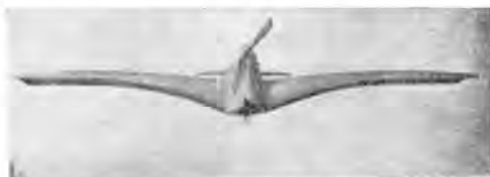
Fig 4b. Guidoni: Monocoque Floating wing with foils
