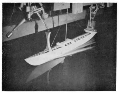
SEA BIRD hull being tank tested.
