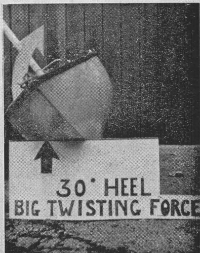
Photo 3. The side view of the model shows the Pitch Pivot Region. The view (lower left) indicates the relatively small reaction of a wave against the bow when the angle of heel is small. When the hull meets a wave at a low angle of heel, the upward and sideways reaction is small. On the right the hull is heeled to 30 degrees, and the large curved arrow indicates that when the lee bow is on its side, it is driven upwards with considerable force by the strong reaction between the waves and the "flat" surface. The bows are also swung to windward which changes the angle of attack of both keel and sails.
