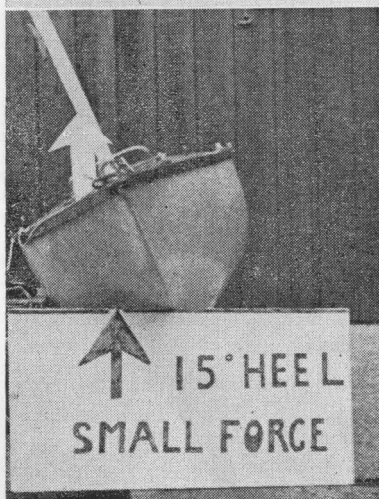
Photo 3. The side view of the model shows the Pitch Pivot Region. The view (lower left) indicates the relatively small reaction of a wave against the bow when the angle of heel is small. When the hull meets a wave at a low angle of heel, the upward and sideways reaction is small. On the right the hull is heeled to 30 degrees, and the large curved arrow indicates that when the lee bow is on its side, it is driven upwards with considerable force by the strong reaction between the waves and the "flat" surface. The bows are also swung to windward which changes the angle of attack of both keel and sails.
