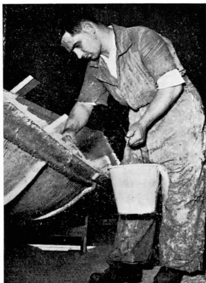
"Layup in female Mould; note stiffeners on mould and mould surplus above sheerline."
