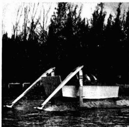
FIG. 8. Miami Shipbuilding's 1/2 Scale LCVP using the Hook Hydrofoil System
