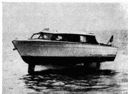
FIG. 18. Gibbs and Cox Incidence Controlled Boat (1957) Foil Borne
