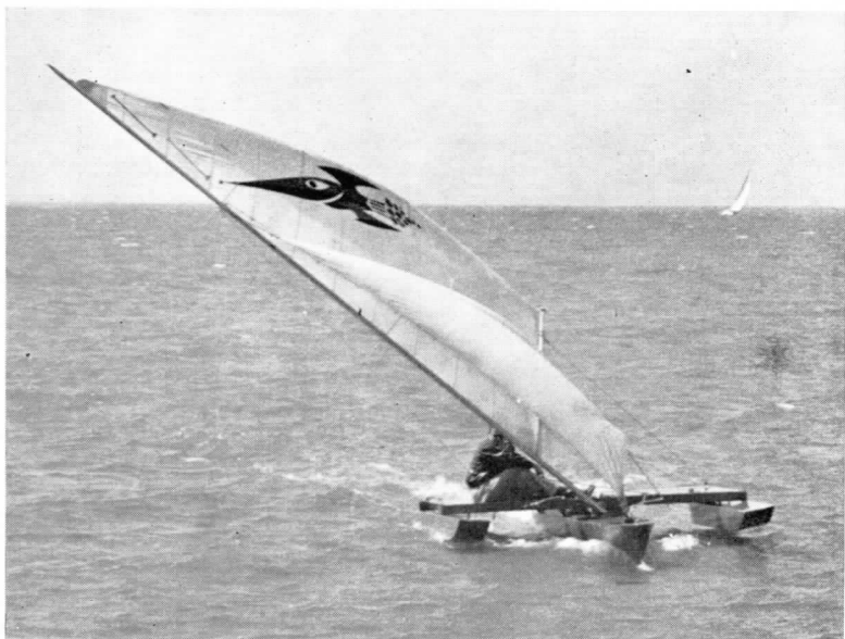
NEW SLANT IN SAILING. Novel tilting rig, which gives lift as well as drive, is tried out on Rocket Outrigger class boat on San Francisco Bay. Designer is Arthur Piver, Mill Valley, California.
