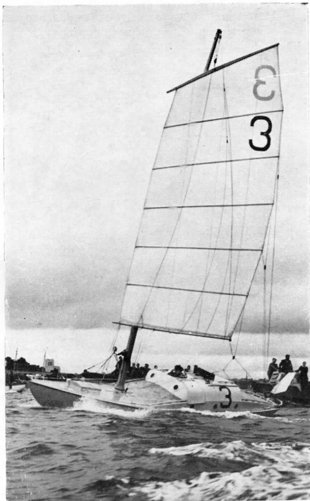
Jester , "Blondie" Hasler's entry with its adaptation of the Chinese lug-sail, had a wind vane that operated a large trim tab on the after edge of the main rudder. 1960. (Photo: Eileen Ramsay)
