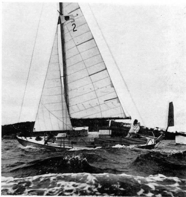
Howell's transatlantic entry also had a wind vane operating an auxiliary rudder in 1960. (Photo : Eileen Ramsay)
