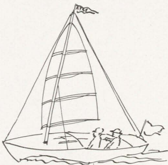
Fig. 11. Semi-Elliptical square-lug-sail with mast stayed to Windward by runners. It could be stayed to lee through Holes in the sail.
