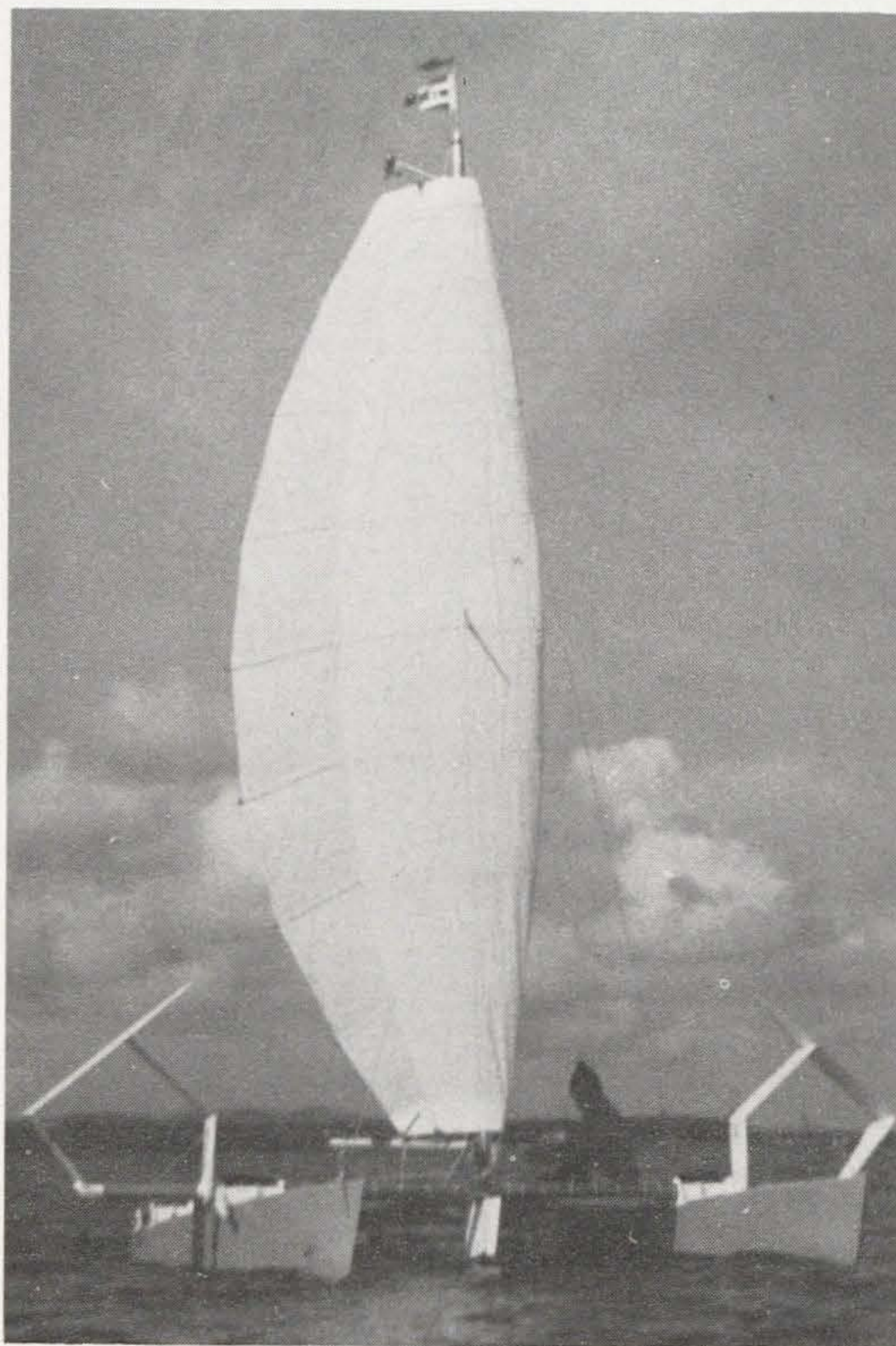
G. C. Chapman's Mk. 4, 10 sq. Metre Wingsail and foils. Raised by rotation about axis of forward cross-beam.
