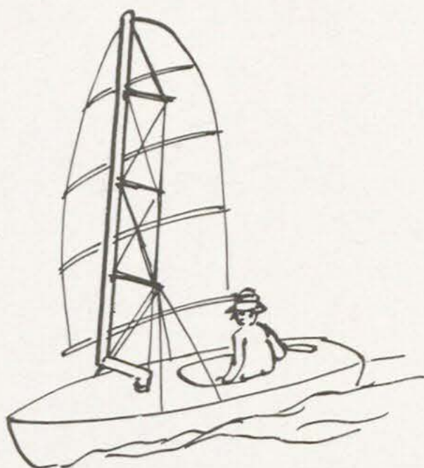
Fig. 10. Crank Mast Rises outside the lee shroud. Staying is to the tip of the lower crosstree.
