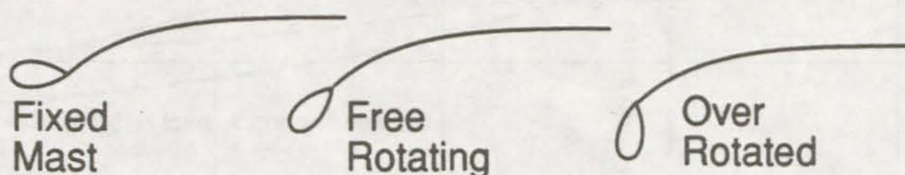
Figure 22 – Only an over rotated mast gives a fair flow onto the lee side of a sail and this increased performance has been demonstrated frequently in practice. Free rotating masts are only slightly better than fixed ones.
