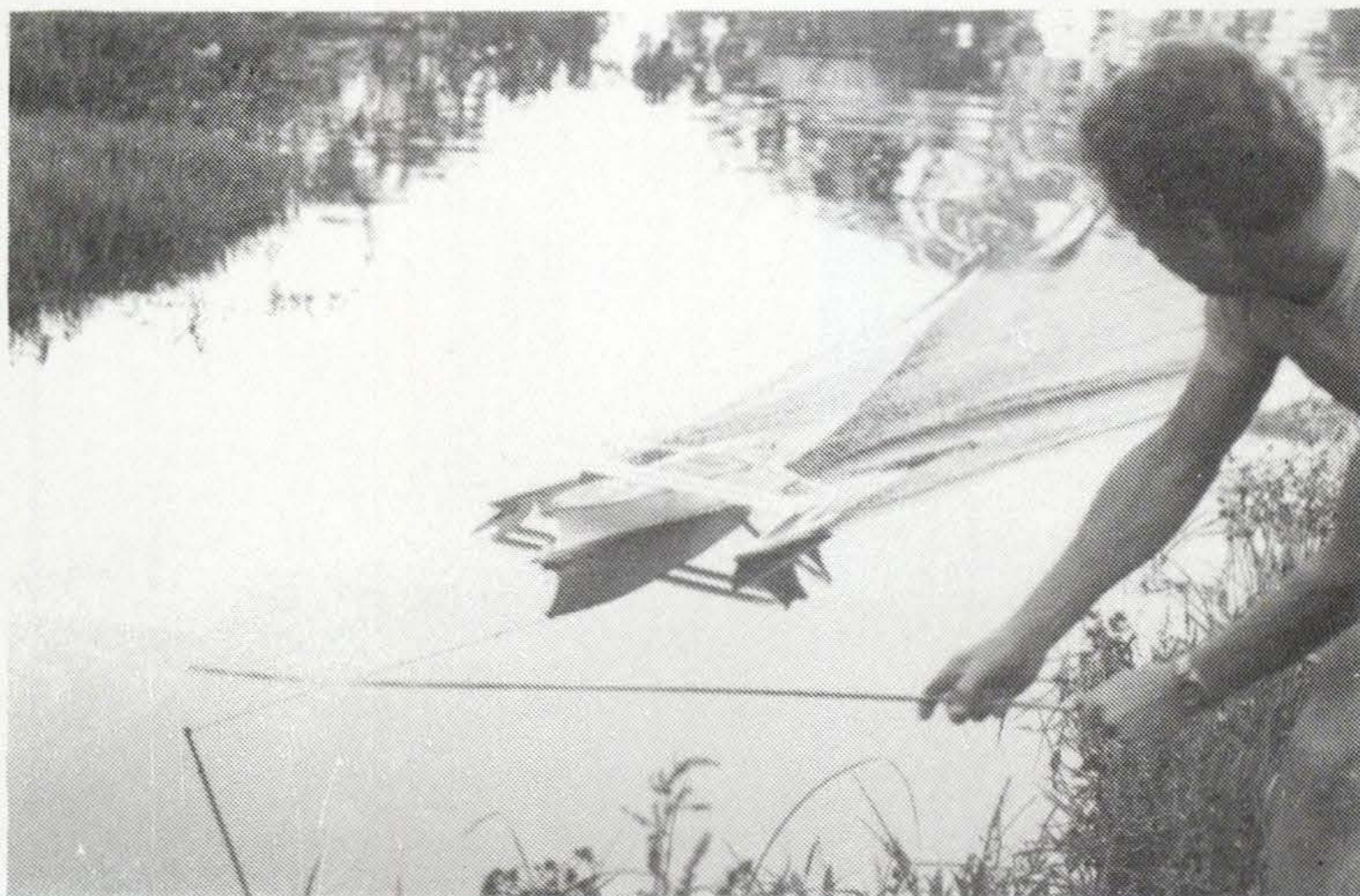
Joseph Dusek testing bulb bows on models. Conclusion = large or small bulbs are best. Advantage = less bow wave + more buoyancy.
