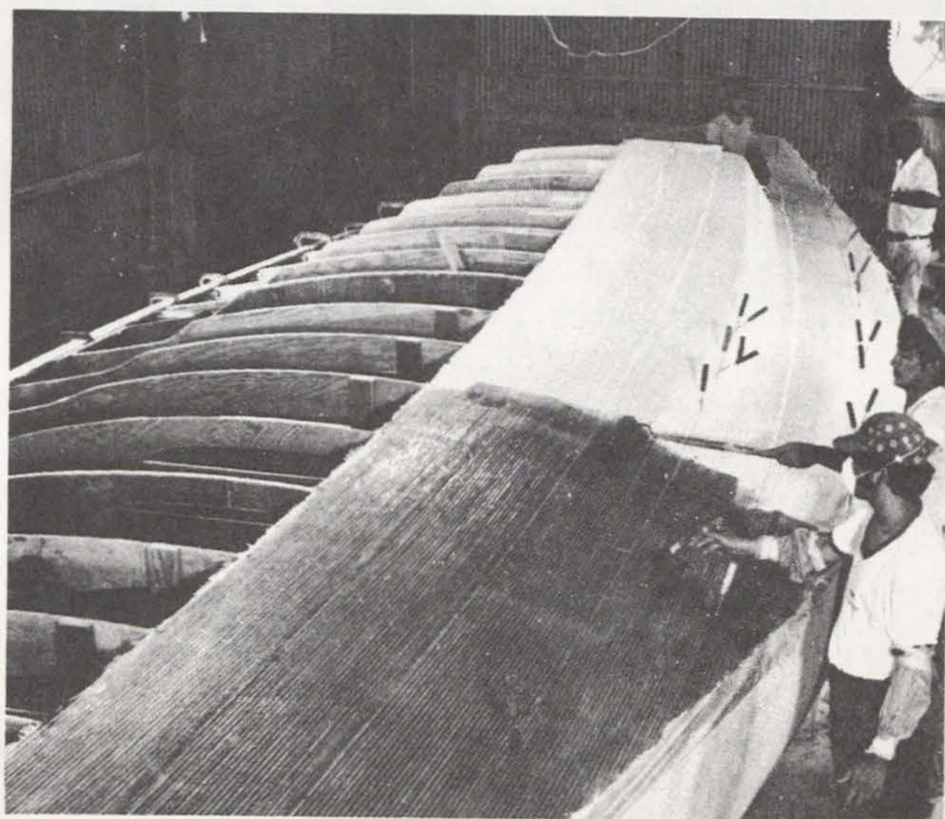
Fig. 11 The Start of a Balsa Core Deck After the C-Flex is in place, it is wet down with resin.
