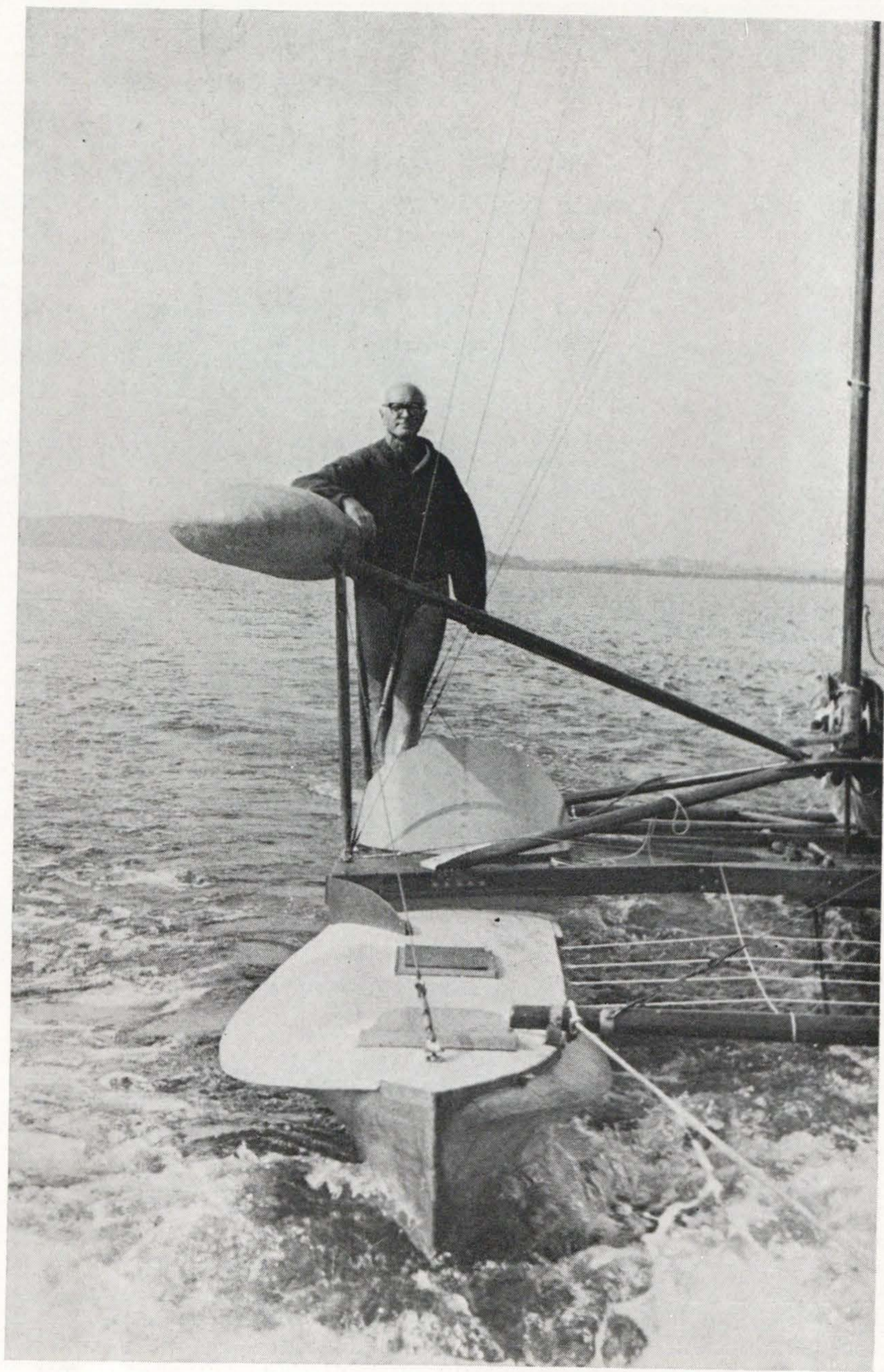
Bow view showing spray deflectors
