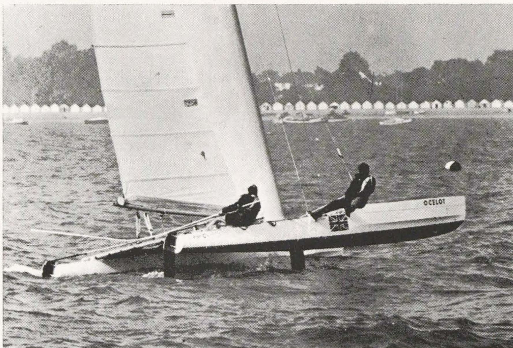
OCELOT . Note deep forefoot and position of centreboard. These made tacking slow
