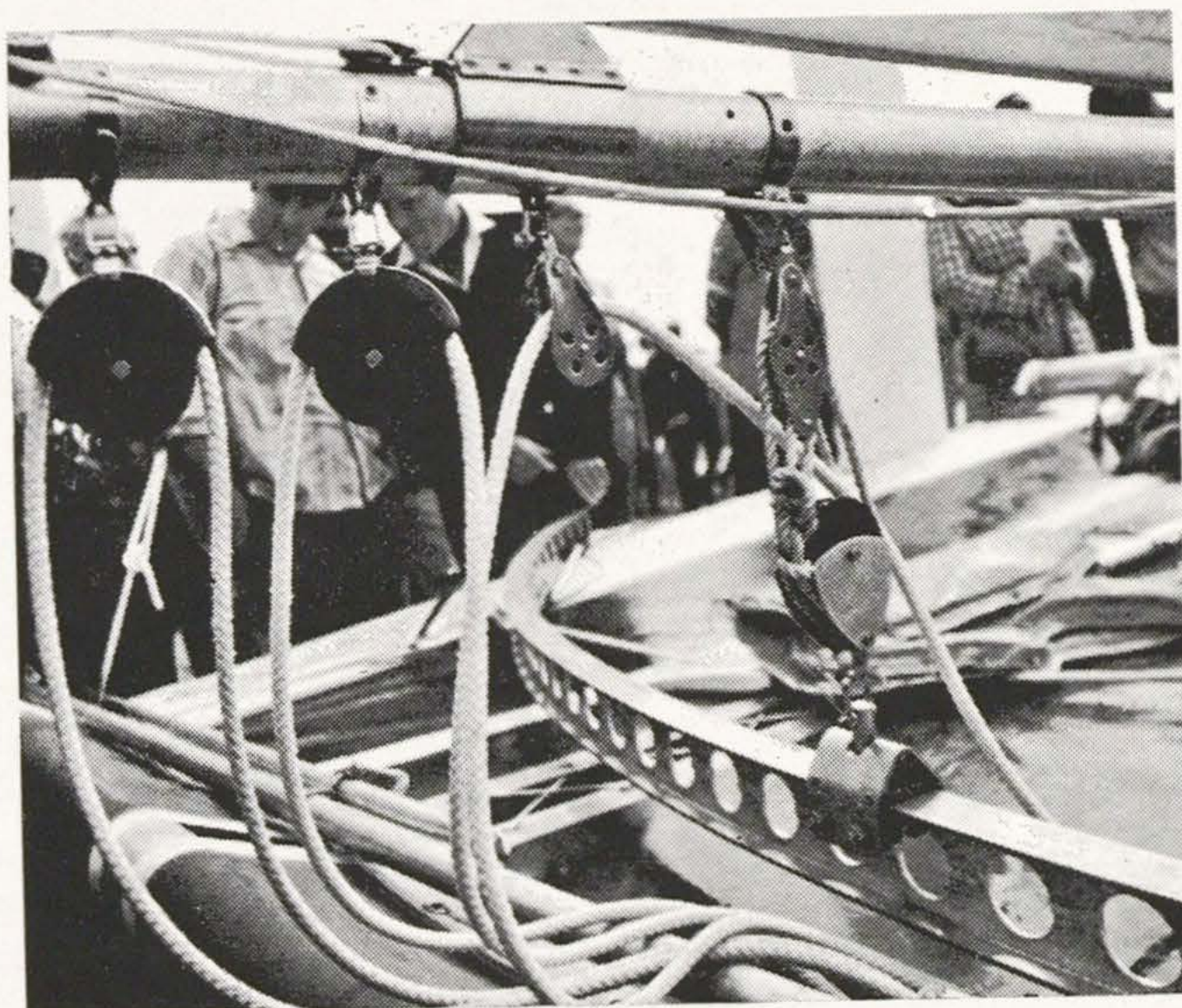
OPUS III's mainsheet and curved, lightweight track Photo: Knights
