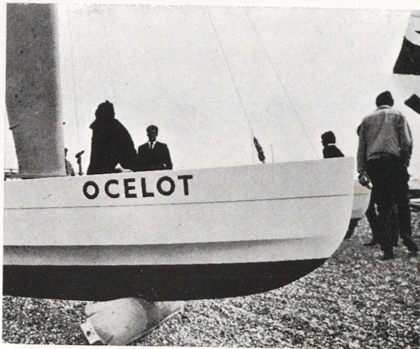
OCELOT's bow showing deep forefoot and knuckle parallel to the waterline Photo: Knights
