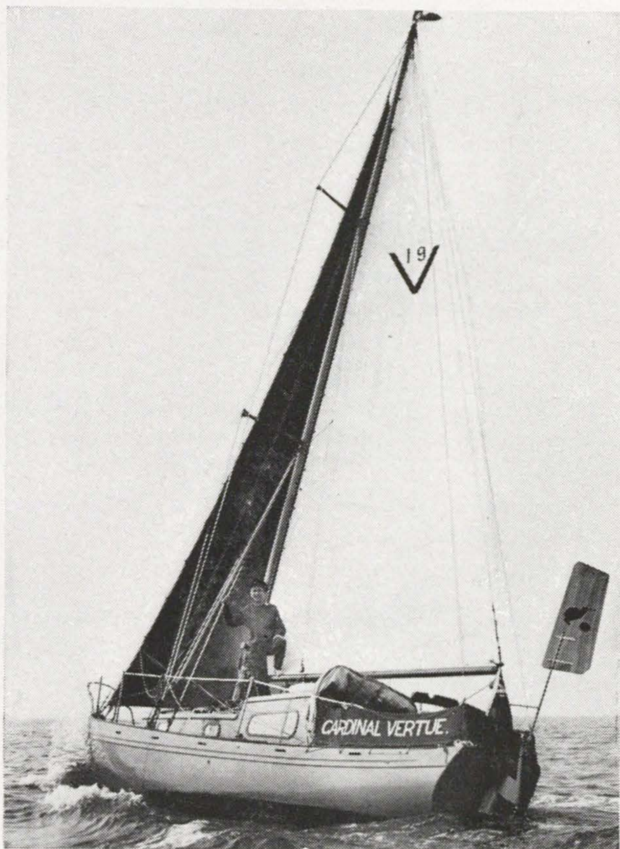
Dr. Lewis's single handed Transatlantic entry Cardinal Vertue had a vane operated trim tab that was really a part of the main rudder. 1960. (Photo: Eileen Ramsay)
