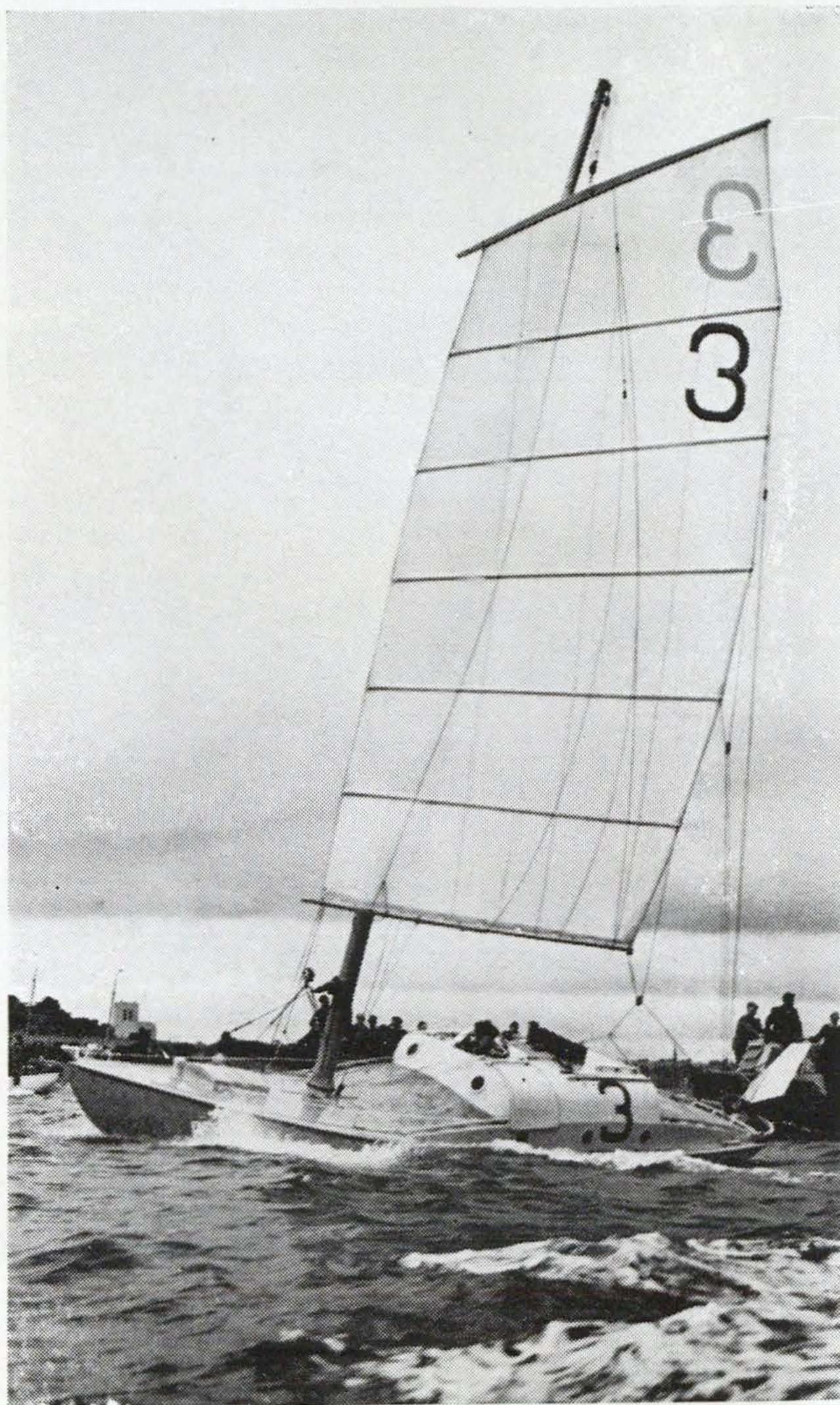
Jester , "Blondie" Hasler's entry with its adaptation of the Chinese lug-sail, had a wind vane that operated a large trim tab on the after edge of the main rudder. 1960.
