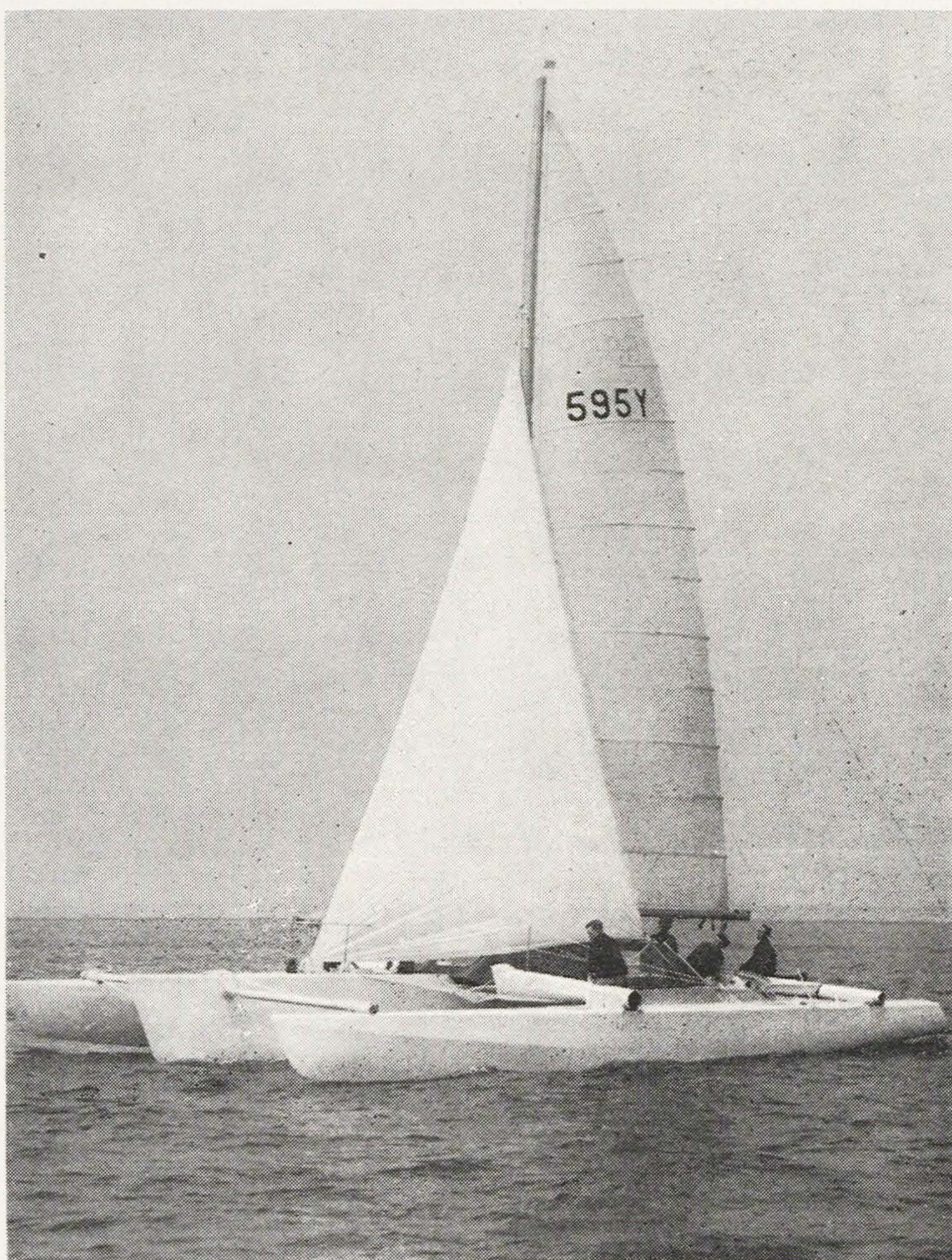
TRIFLE, a fast and relatively trouble-free trimaran designed by Derek Kelsall for Maj. Gen. Ralph Farrant. She is built of foam plastics, covered with glass fibre.
