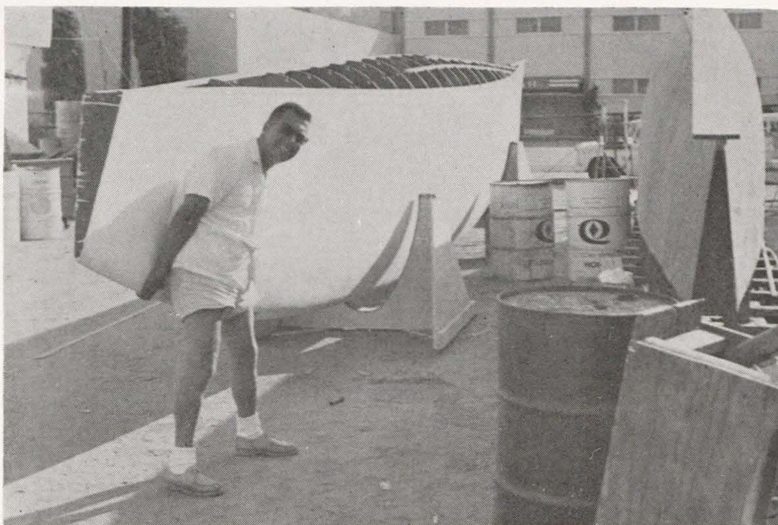
SEA BIRD hull being lifted to show light weight.
