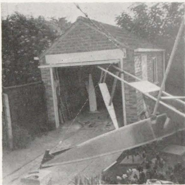
Martin Sanderson's hull, cross beams and forward steering foil with "feeler"
