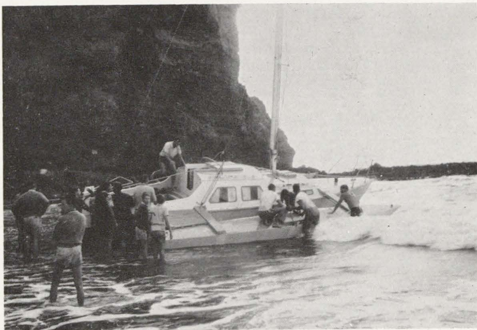
TOLU VAA on Piha Beach. Nearest float full of water and missing side deck.
