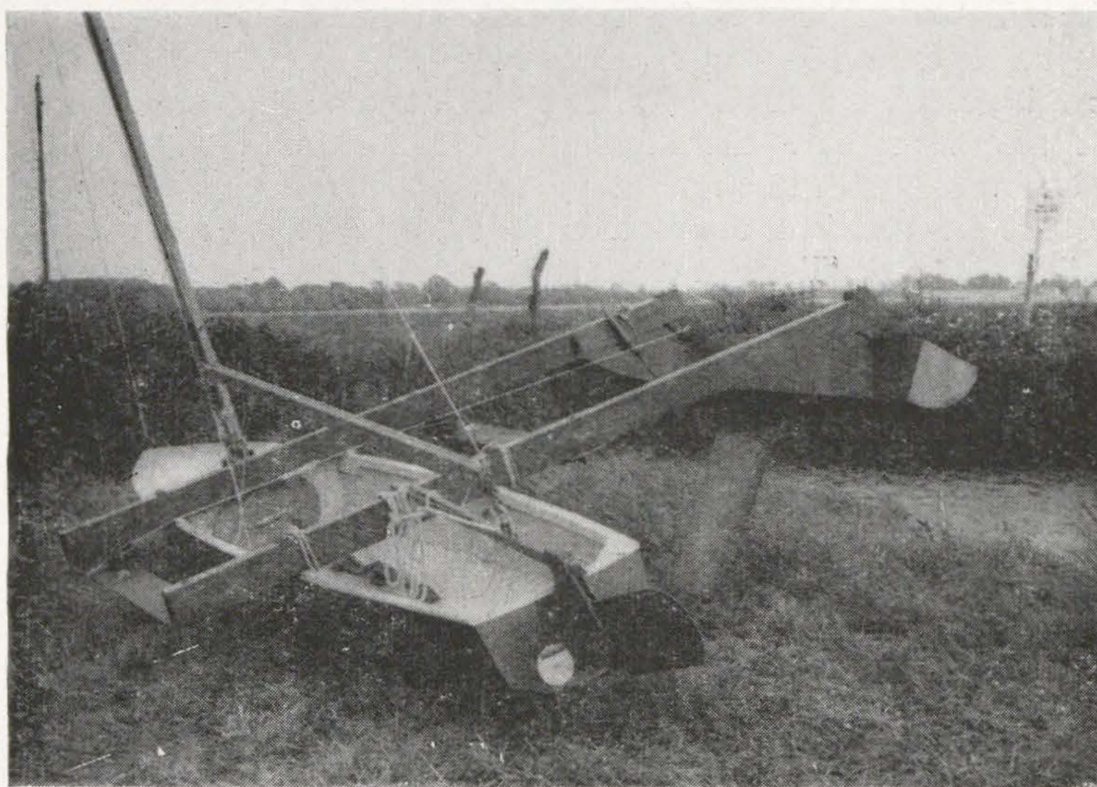
TRIPLE SEC showing cross-arm mounting
