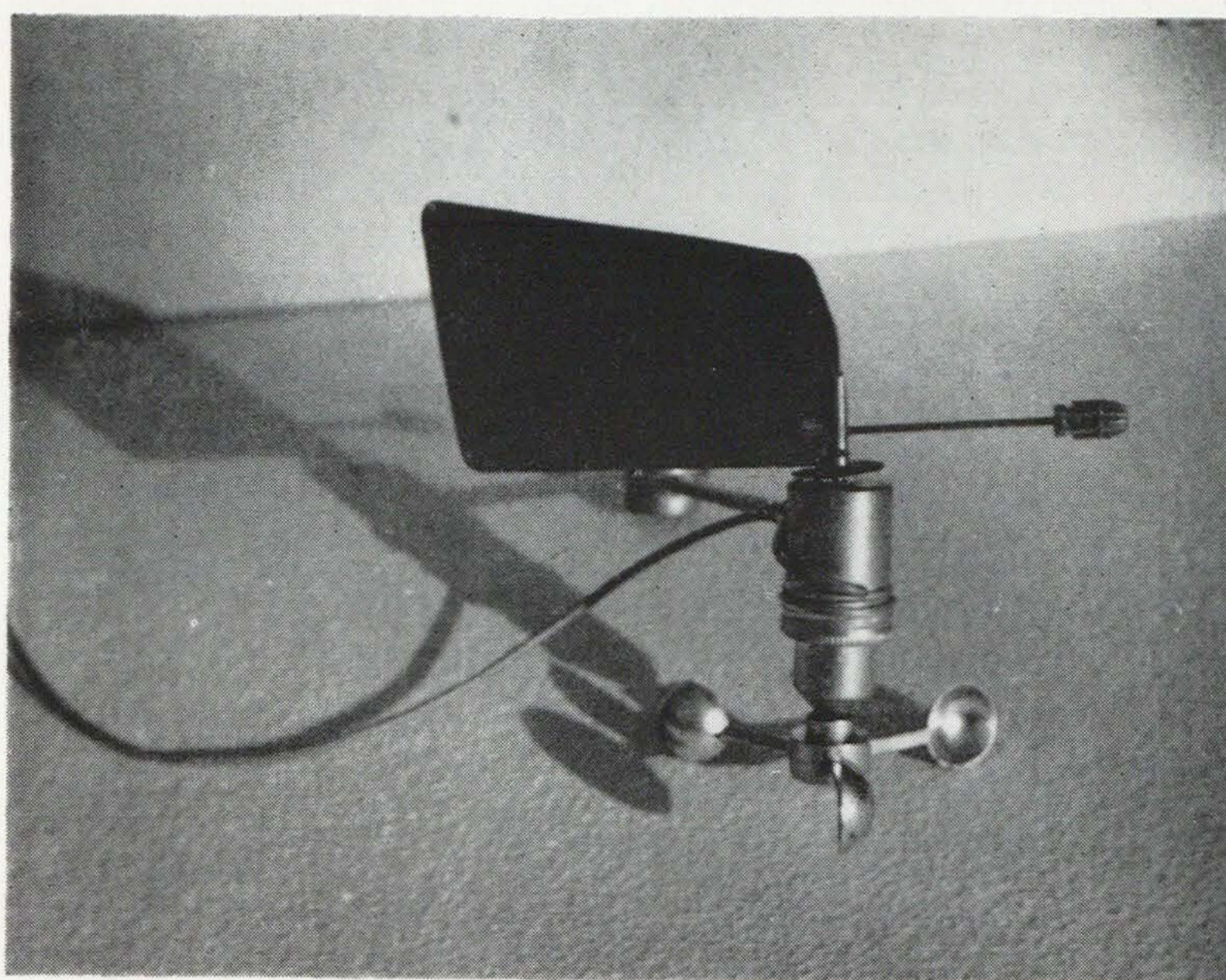
Vane and cups for wind angle & speed
