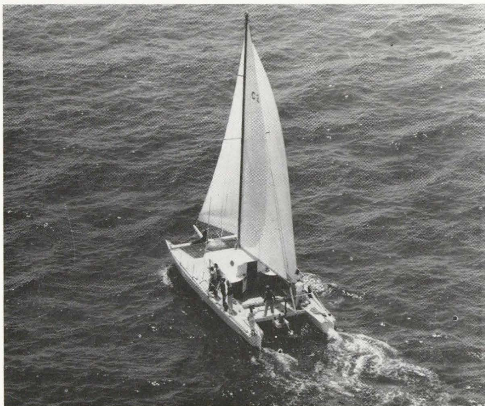
FIG. 8. The 43-foot Dreamer , third largest active cat in southern California, has flared symmetrical hulls and 18-foot beam, giving her great reserve buoyancy and carrying capacity (she recently carried, fed and slept fourteen people for three days). Her dagger boards and Watts racing jib give her good speed to windward.
