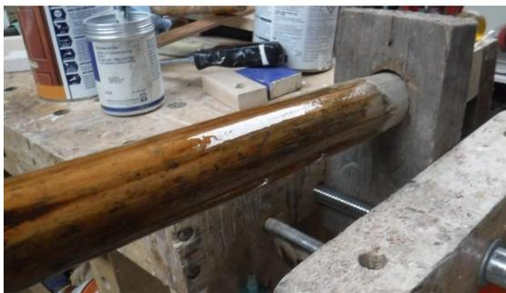
Nothing special just how I support my oars when recoating them. Just a block of wood with a hole that loosely fits the handle (left uncoated for grip) held a bench vice so that the loom is just sloping up from the horizontal, it is then firm, but by working outwards one can easily lift the loom a little to rotate it as you apply the finish, eventually reaching the tip of the blade and the very last bit you do without being able to rotate. Wear gloves to avoid skin grease and
