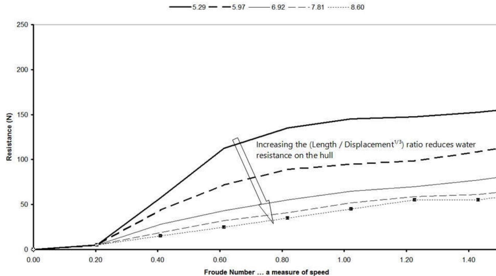
Chart is for hull type "series 62 single chine" with test data collected by Clement & Blount 1963
