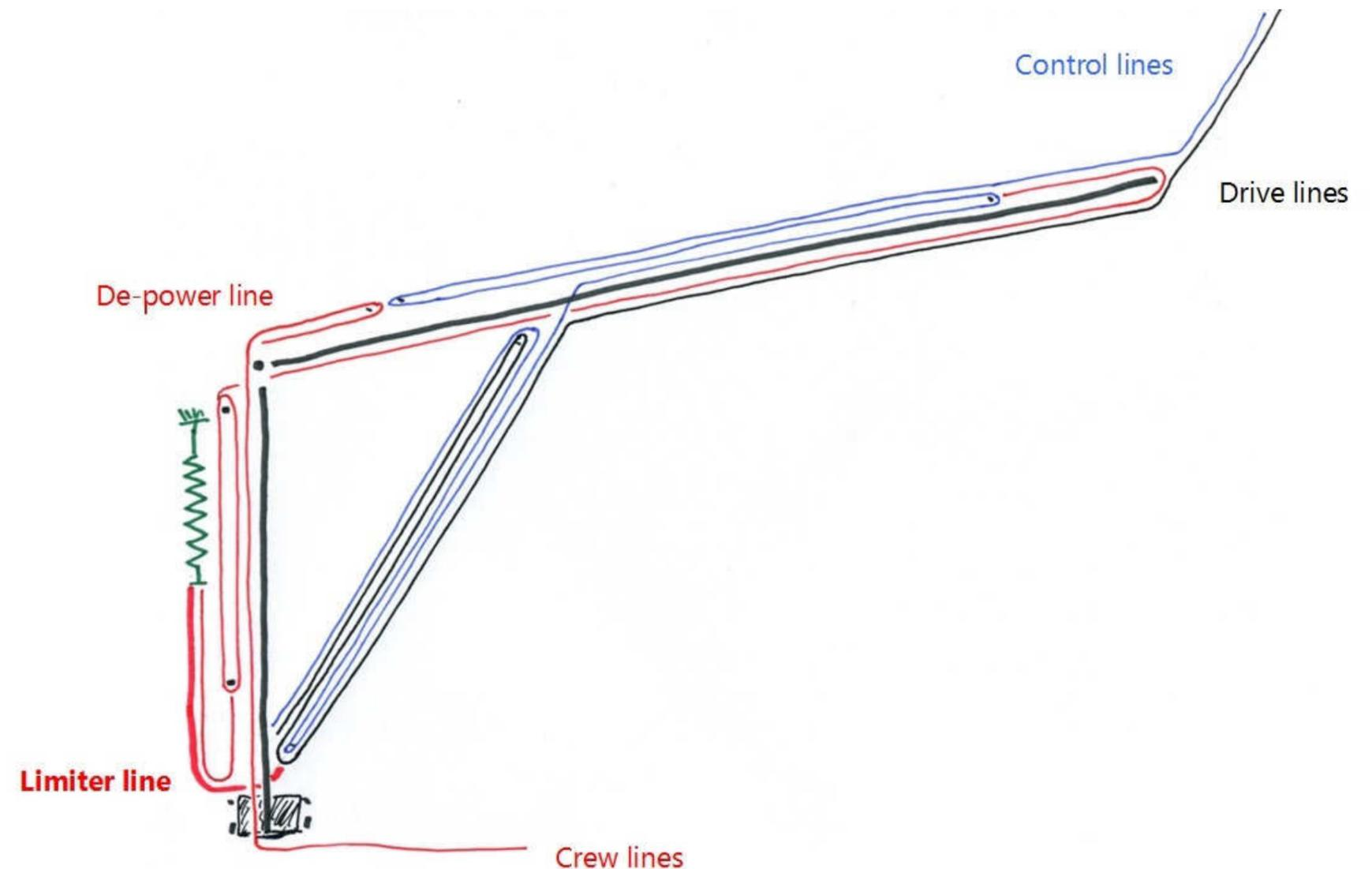
When the selected maximum kite load is exceeded the spring extends. The 'load limiter line' therefore extends which moves the pulleys at the end of the boom. This increases the length of the 'control lines' and depowers the kite. This arrangement allows the control lines to be used to control the kite as the spring extends to depower the kite.
