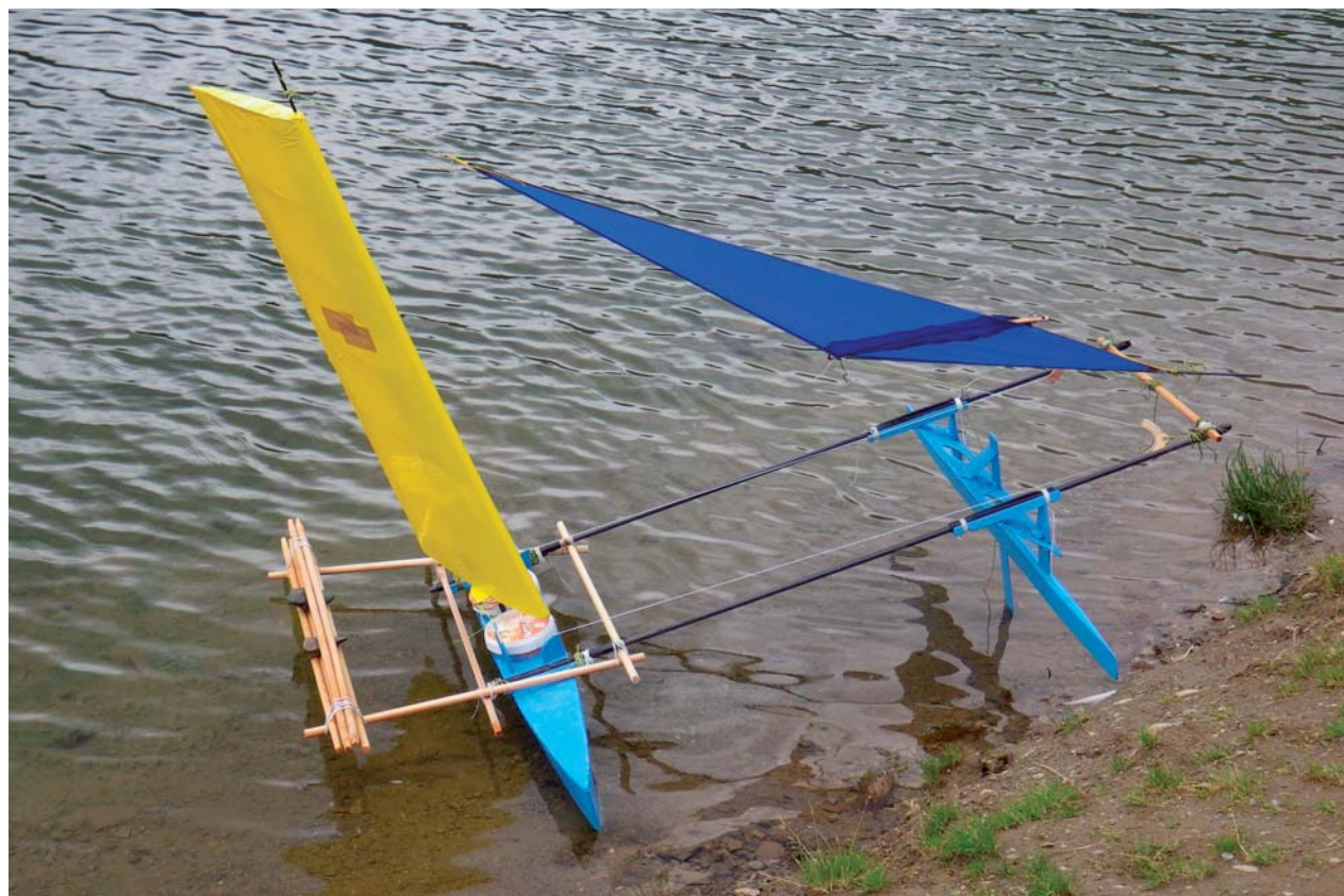
Figure 4. Model proa Norwegian Blue. The blue jib seemed to contribute most to driving the boat, while the yellow wing was used primarily for steering. The leeward counterweight was needed because of the small volume and high density of the solid wood windward hull.
