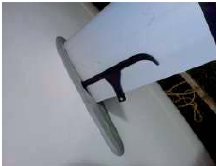
Wand retracts neatly within the centreboard
