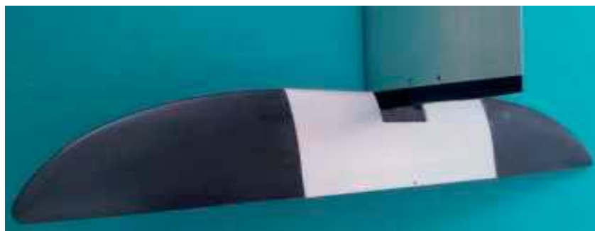
With flapless foils, the entire foil rotates. There is no flap and no joints across the foil to cause drag
