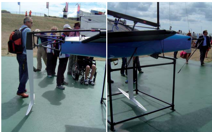
Moth - rear foil, main foil and wand
