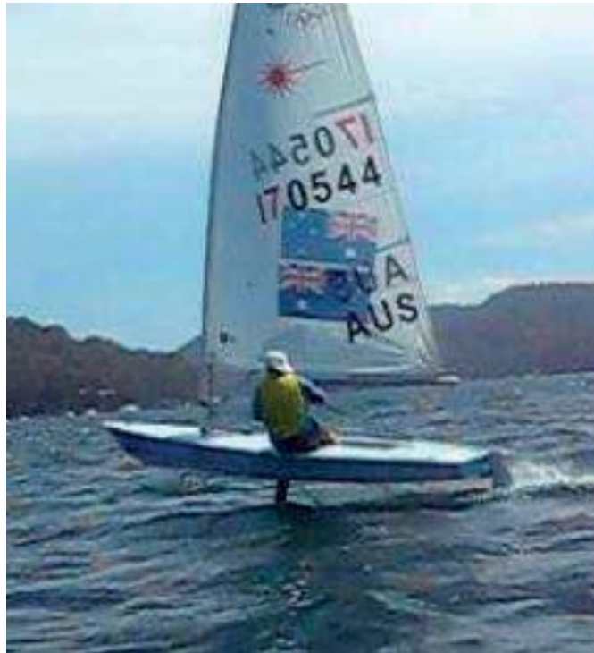
World's first foiling Laser, using centreline foils in 2010
