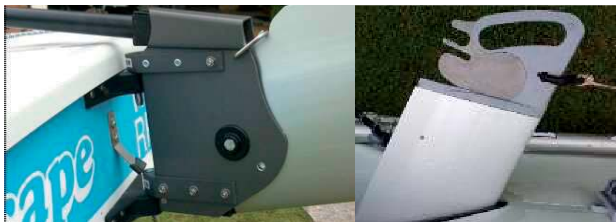
Retractable rudder & centreboard makes rigging and launching in shallow water simple
