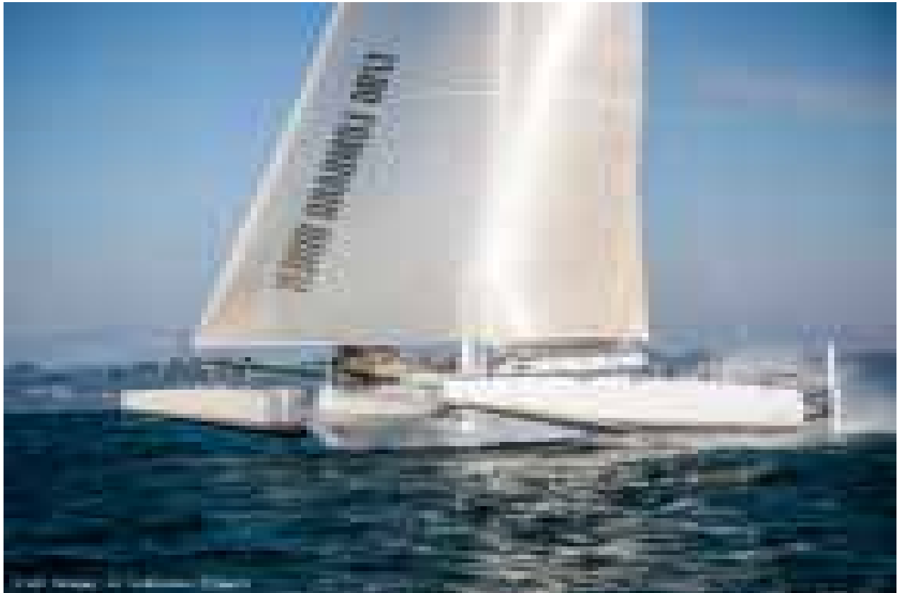
l'Hydroptère.ch, the holder of the main speed records on Lake Geneva, is the Hydros project's flagship vessel. Note the retractable planing steps under the hulls just forward of the foils. Photo: Copyright ADimages-A_Tinturier
