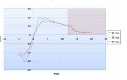
Cl/Cd vs AOA for NACA 0012 Airfoil – Aspect Ratio 2:1
