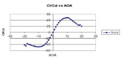
Simulated Cl/Cd curve for a NACA 0012 Airfoil
