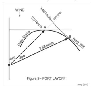
boat's velocity is increased to 3.68 knots. The velocity made good towards the target increases to 3.46 knots, a gain of 0.55 knots, or 19%.
