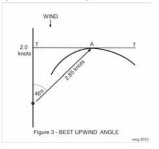
remote place, while points to the left mean the boat is "pinching" – heading closer to the wind, but moving slower.
