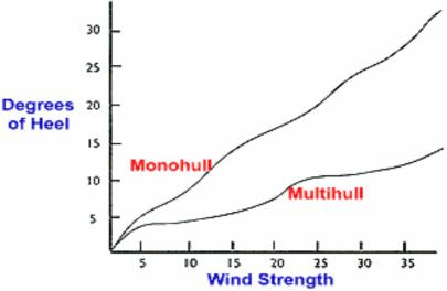
Figure 4: Graph plotting degrees of heel against wind strength for a mono and multi hull boat
