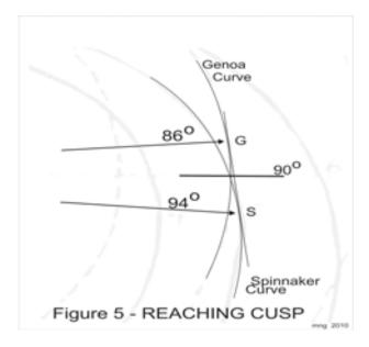
The reaching cusp is clear of the centreline which is the core of the upwind and downwind cusps. So this cusp is not symmetrical. The two cheeks come off at different angles. Also, these angles vary with wind-speed. Here is a detail of the one at 5 knots. We see the cusp occurs at 90° course angle. (An enlargement of the centre of this figure is Figure 6).
