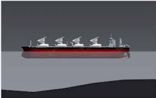
Figure 3: At sea in favourable conditions, the module doors open temporarily to allow the masts and sails to extend upwards, and the doors then close around the base of the extended rig.
