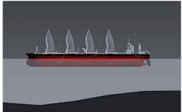
Figure 4: The extended rigs provide sail assistance to the ship, allowing it to throttle back its engine.
