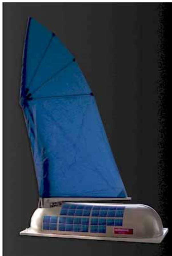
Figure 11: pod closes around extended rig, and the mast and boom rotate into the correct position for sailing
