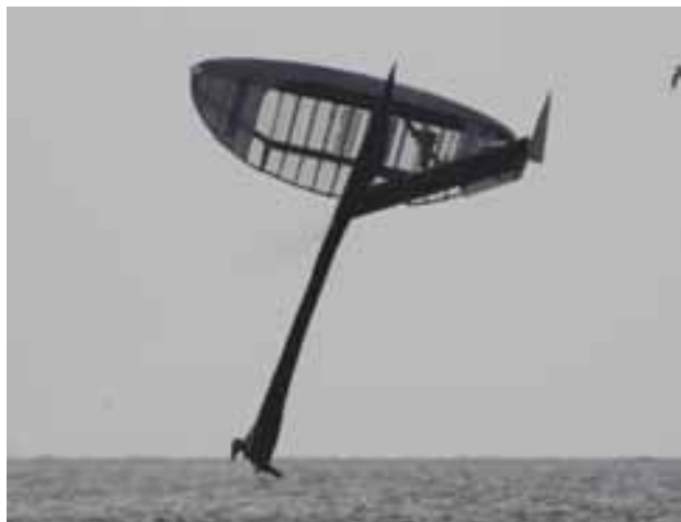
At this point, a few seconds later, Sailrocket is very much a glider without a tailplane. The wing is still lifting the bow, but there is no lifting area aft to balance it. Now there is no way out of the flip.
