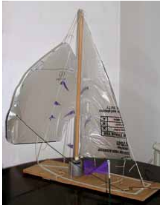
Figure 1. Smaller model rig, “wind” coming over port quarter. The dark chiffon strips are wind tell-tales.
