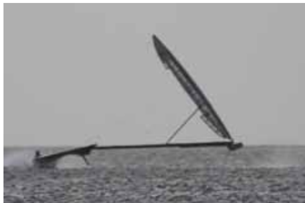
This is the beginning of the first flip, in Oct 08. The bow has just lifted off, the foil is out of the water, and there is nothing to counteract the lift of the sail/wing except weight (Both photos by Helena Darvelid)
