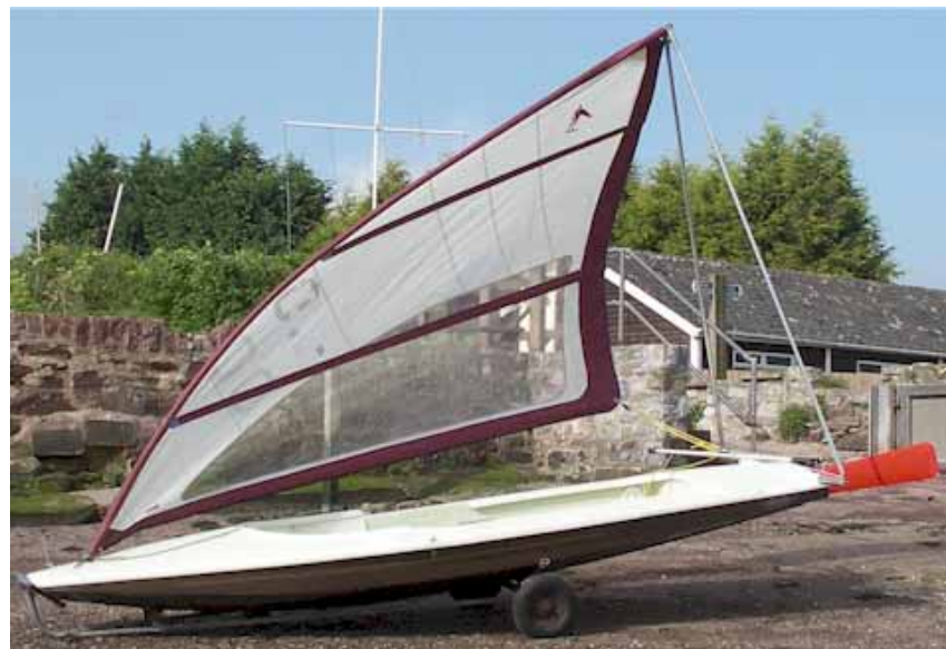
Figure 2: Sail filling and lifting due to airflow across it
