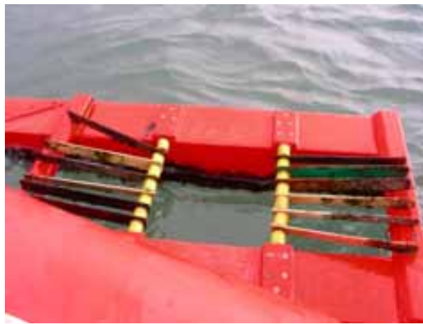
The float at recovery time, steel strips raised
