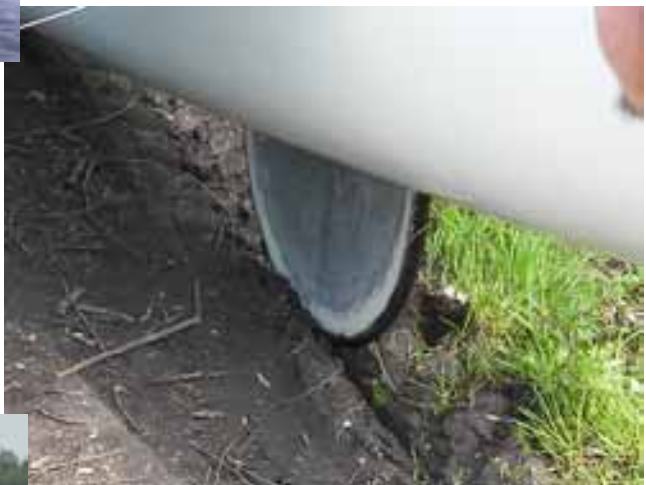
(Left) Alex Stanley's wheeled catamaran and (below) details of a wheel. One of these fits into a cassette in each hull. The wheels themselves are made of two shallow FRP cones with a solid rubber tyre. The cassette allows them to be removed (downwards) for maintenance. As far as one could tell, the performance was not significantly worse than any other catamaran with keel or dagger board, whilst the wheels allowed Alex to land his boat on the slipway and be off whilst others were still looking for their launching trolleys!
