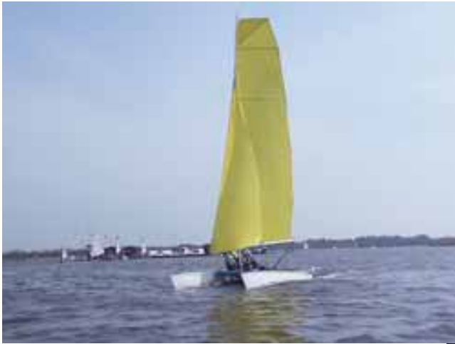
(Left) Alex Stanley's wheeled catamaran and (below) details of a wheel. One of these fits into a cassette in each hull. The wheels themselves are made of two shallow FRP cones with a solid rubber tyre. The cassette allows them to be removed (downwards) for maintenance. As far as one could tell, the performance was not significantly worse than any other catamaran with keel or dagger board, whilst the wheels allowed Alex to land his boat on the slipway and be off whilst others were still looking for their launching trolleys!
