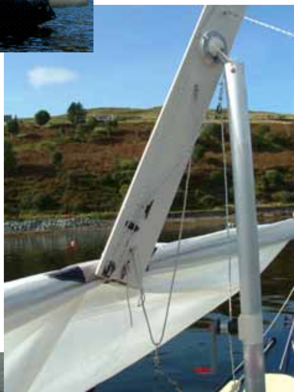
Photo 4 - lower end of halyard arrangement prior to hoisting sail - after hoisting, cam cleat on cross-spar holds halyard while turning block is unclipped from masthead and clipped to eye on cross-spar - halyard is then made off on cleat on cross-spar.
