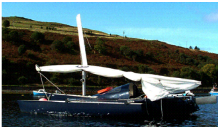
Photo 3 - sail rigged ready to hoist - see 'nose' hinge at forward end.
