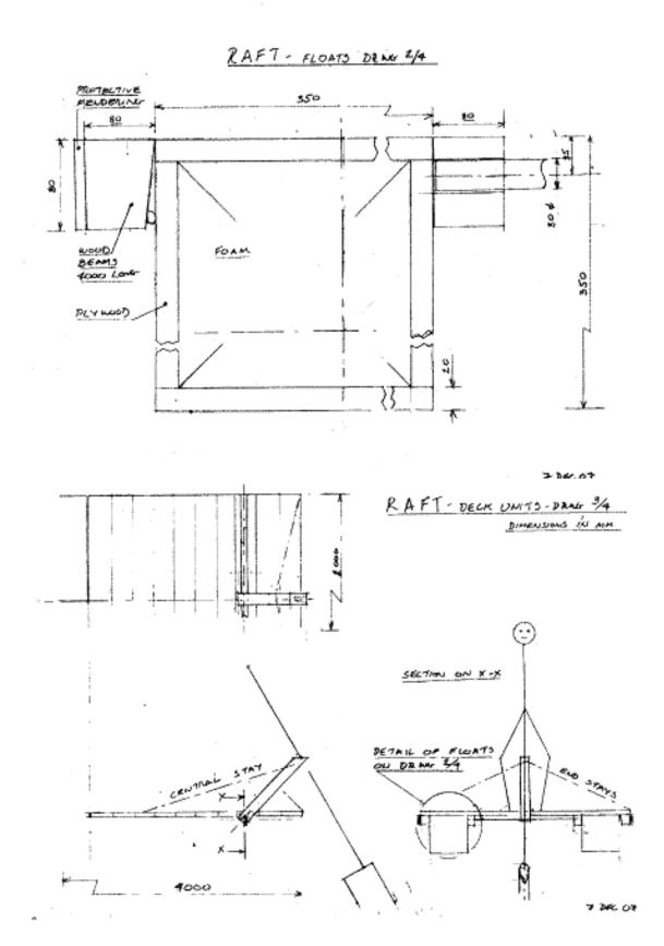
(i) Two hollow plywood floats 4 metres long and of 35 cm '35 cm section, shown in drawing 2.
