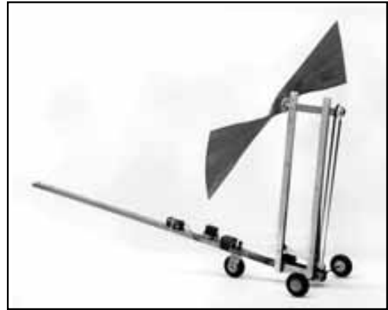
The wind car in its' short and narrow 'treadmill' configuration. Note the radio control for steering and brakes. The mast with apparent wind flag is not shown.
