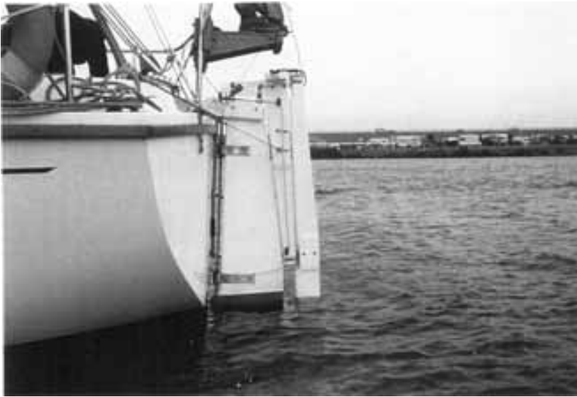
Fig 6: The prototype oar and oar carrier made from plywood
