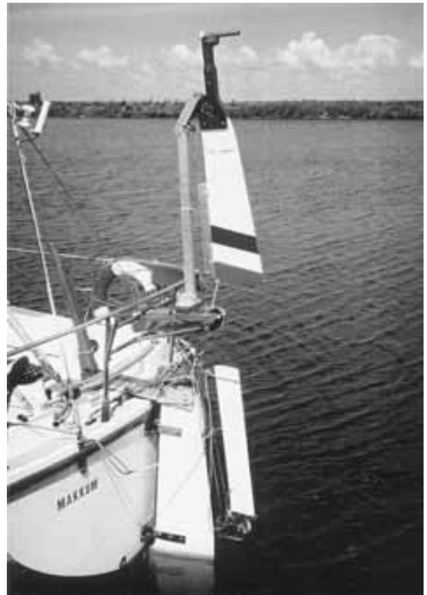
Fig 8: The oar blade retracted
