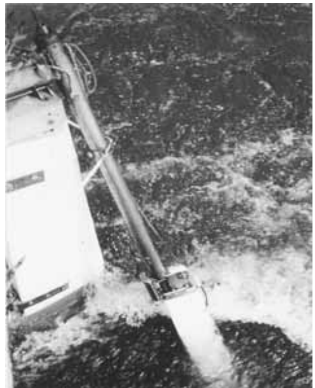
Fig 10: the oar working out of the rudder wake
