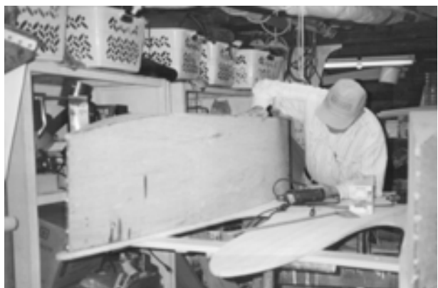
The Mini-Trimaran III is made of plywood and fibreglass.
