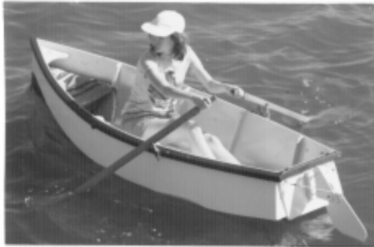
Cindy Darby Tucker rowing the Darby SS 8. Note the kick up skeg which helps it go straight. This skeg is removable.
