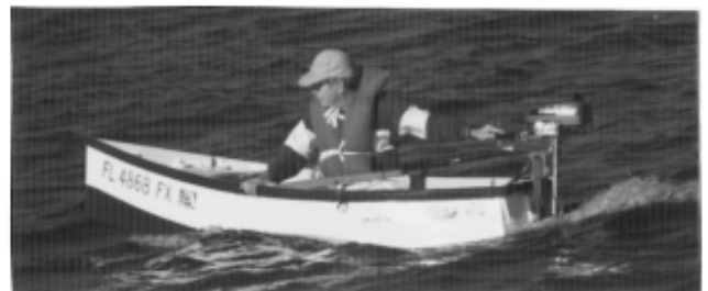
The Darby SS 8 powered with a 1.5 H.P. gas motor. It also handles well with electric motors and can operate in less than 8 inches (20 cm) of water. It can operate in much shallower water than most PWC jet boats at slower safe speeds.
