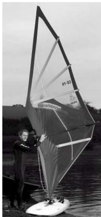
Figure 8: a windsurfing rig using significant areas of transparent stretchy film.
