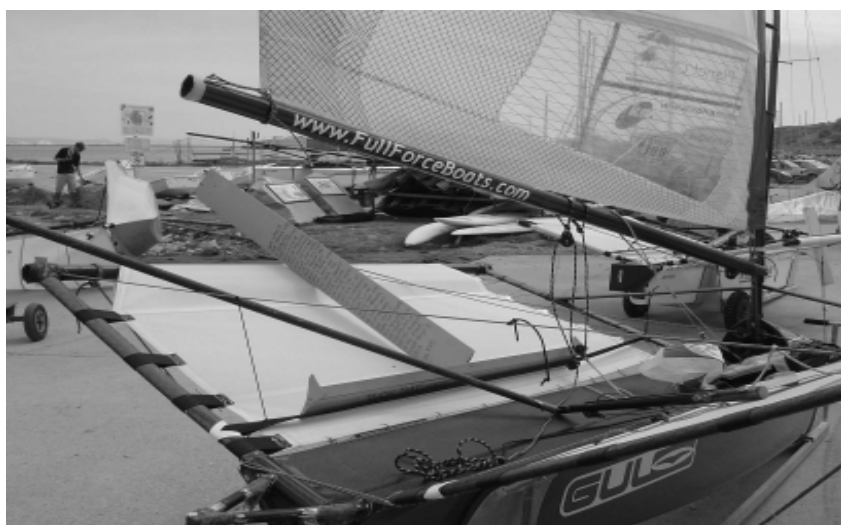
Graham Vial's Moth: homemade foils - note small end plates. (Photo: Chapman)
