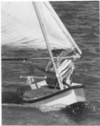
When sailing the Darby SS 8 it is easier to keep up-right than wide dinghies with centerboards because the sailors can shift their weight on a narrow hull more quickly and there is not a centerboard well in the way in case of a strong wind shift.
