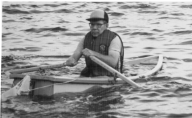
In this picture the boat was deliberately filled with water to show how it keeps afloat. It is designed so all the water shown in the boat here can be spelled out in seconds in deep water and the sailor can roll back in easily without bailing.
