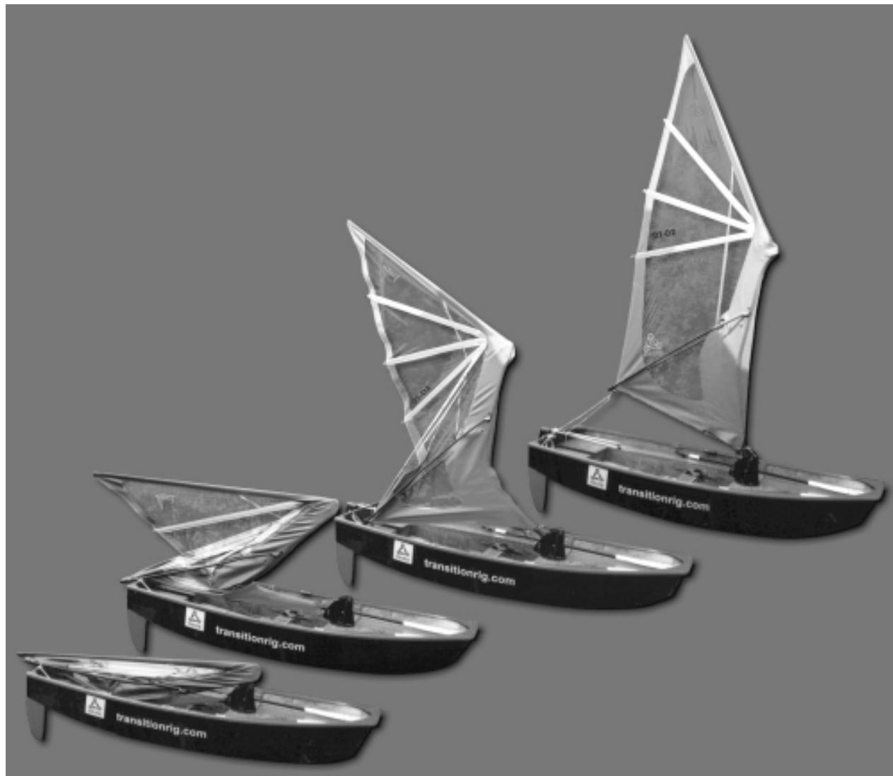
Figure 9: composite picture of the dinghy version showing folding of the rig.
