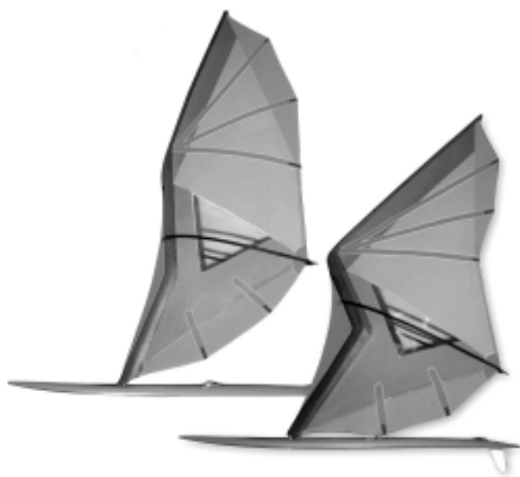
Figure 7: on the left, the rig is fully extended as it might be in a light wind, and on the right it is more flexed in response to a stronger wind.
