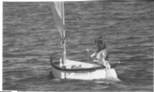
The lateral resistance designed into the hull allows this boat to tack up wind without a deep daggerboard or deep rudder. Because of its small size it can jib by swinging the boom over the bow like windsurfers do.
