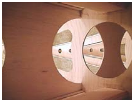
Figure 5-47 Plywood shear webs join the leading edge skin and upper and lower spar caps. Lightning holes are cut in the shear webs. Note the distance between the rear of the spar cap and the shear web. This is because this is the lower section, and the stub-mast will fit just inside the circular opening in the rib. After the load test, the spar cap was extended back to the shear web and the shear web reinforced with thicker plywood.
