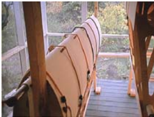
Figure 5-46 Plywood leading edge skin glued to wing ribs. The wing skins suffered severe cracking problems when bent around the leading edge. In order to accommodate the sharp radius of curvature, the wing skins were thinned and soaked in water before gluing them on to the ribs to form the forward “D” tube. This area remained weak and prone to damage in the finished wing structure.
