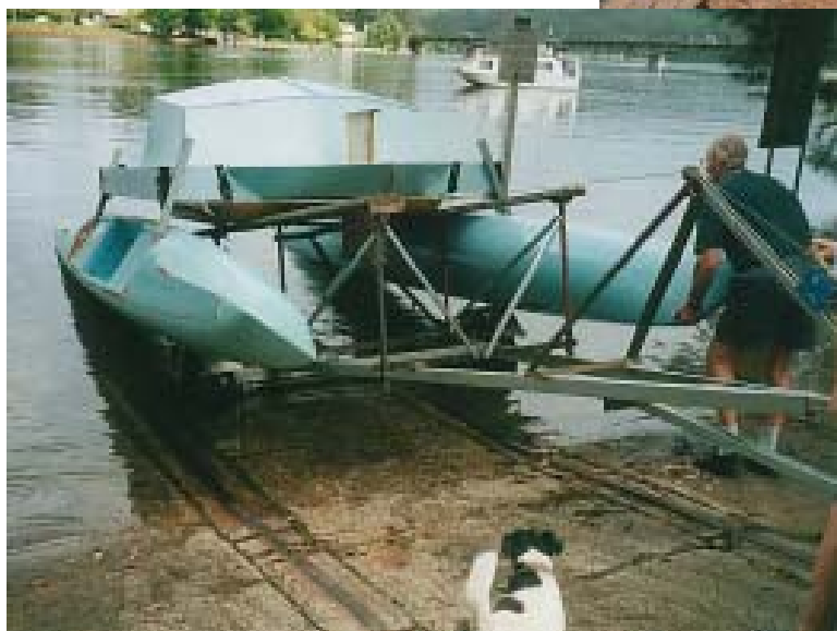
Photo 5 (above) - the cat is carried on its trailer with the hulls folded under its bridgedeck so that its beam 2.5m, the legal maximum towing width.
