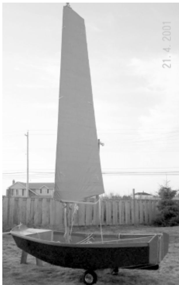
Figure 1. A cheap junk wingsail of 24 sqft on an 8 ft pram. Wind is coming across port side and the wing has feathered into it.
