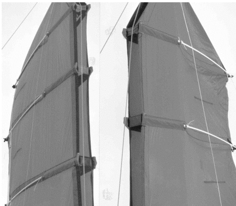
Figure 9. The internal spreaders go through the sail to the battens just behind the ends of the short batten pockets. To get rid of the sharp kink on the weather side, the batten pockets could be extended beyond the spreader a little, and flared out gradually. The mesh covering the front opening is not clearly visible in this picture.
