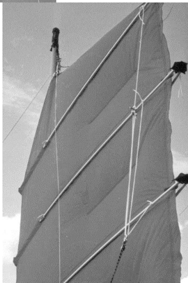
Figure 10. Internal fabric ribs prevent the sail from getting baggy when feathered.
