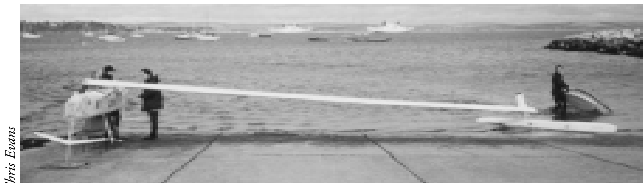
Dr. Guy Hawkins and his team assembling his exotic craft for the first time. A very well built proa that had people guessing for days as it stood in the car park on its trailer waiting for calmer weather to begin the first assembly. There is a rudder at each end which is designed to 'castor' when the craft is shunted. The cross beam is free to swing and the understanding is that it will find its own point of balance.
