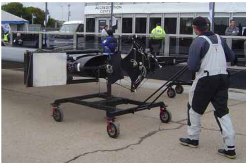
The bottom of Team Korea's wing. The white square is the counterweight tank of water used to balance the wing when hoisted by one of two cranes that come with the circus
