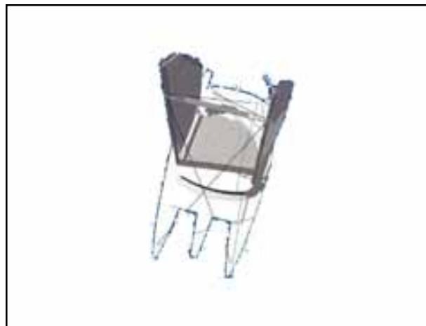
KSS Kittiwake 42 – stays arrangement for a Kelsall Cat Rig.
