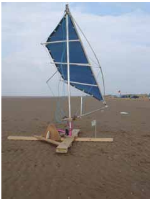
MORLEY Tethered Kite Sail - Static Demonstrator “flying” in a 12 knot Southerly breeze on Ainsdale Beach, Merseyside - 18th April 2011
