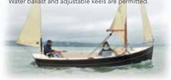
Above—Swallow Boat's Bay Raider 20, a water-ballasted yawl. For more information, see www.swallowboats.co.uk/content/view/115/110
