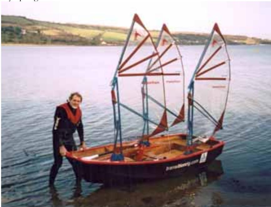
*Figure 14: three transition rigs mounted on a Mirror dinghy*
