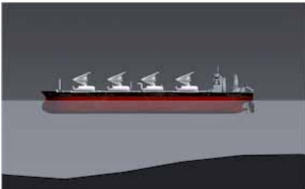
*Figure 3: At sea in favourable conditions, the module doors open temporarily to allow the masts and sails to extend upwards, and the doors then close around the base of the extended rig.*
