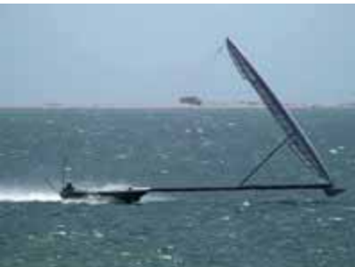
and Sailrocket (Reached ~52 mph at ~21 wind ? so far; \eta \sim .00083 ?)
