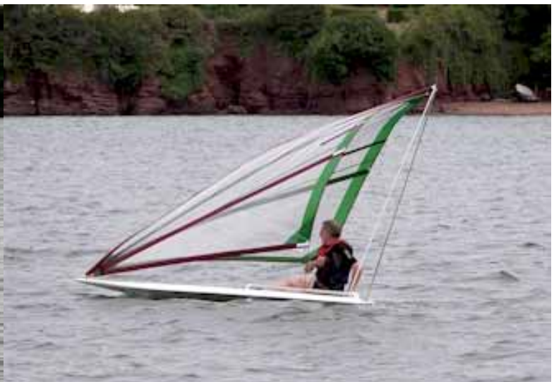
Figure 7: Flèche going down wind with the sail laminae separated
