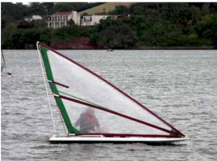
Figure 6: Flèche going upwind with the sail laminae together
