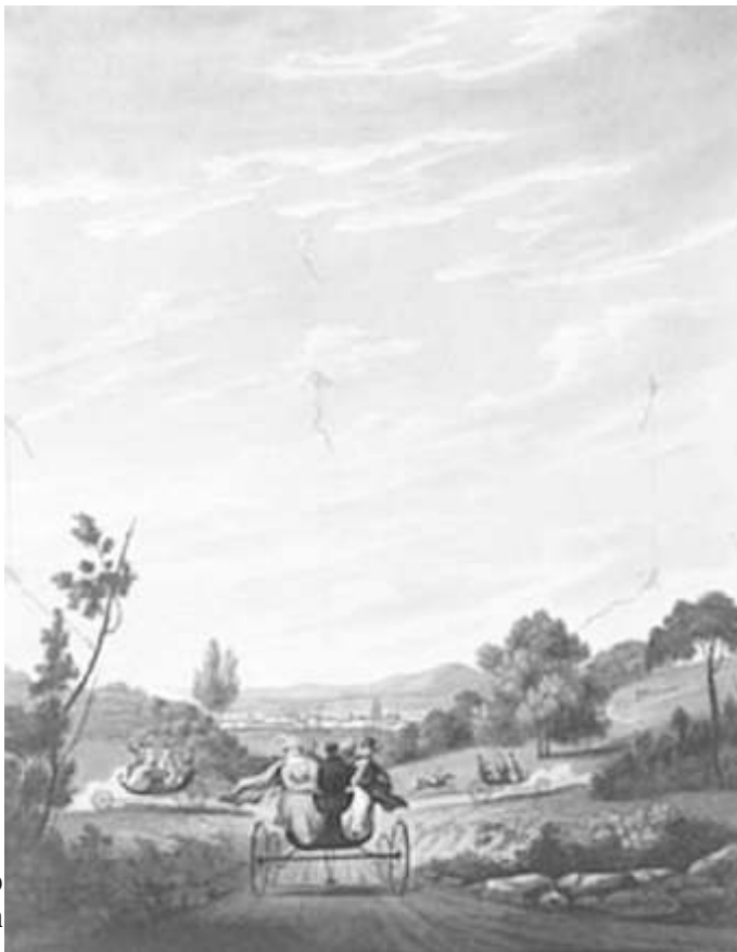
Three Pocock char-volants pulled by kites travelling in various directions, eg tacking with the wind
