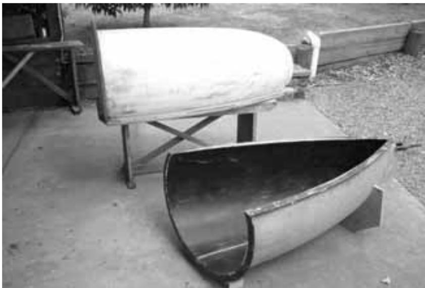
*Photo 10 - plug and mould for Centrehull.*
