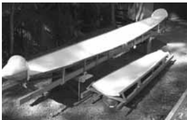
Photo 6 - mould setup for laminating a full length half hull of WRC6800. The deck mould is on the right.
