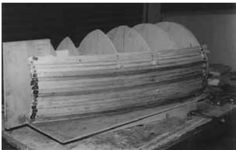
*Photo 9 - Strip-planking the Centrehull plug with 10x20mm timber.*
