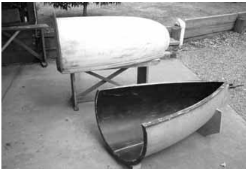
Photo 10 - plug and mould for Centrehull.
