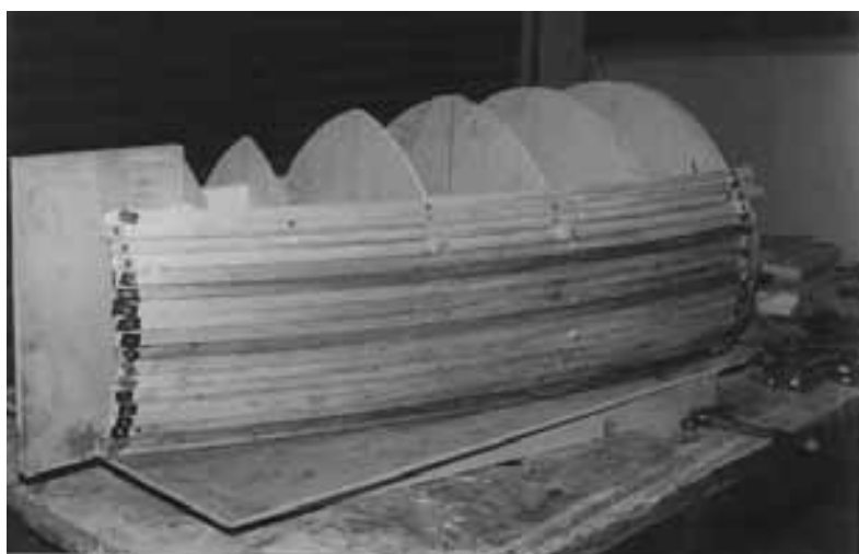
Photo 9 - Strip-planking the Centrehull plug with 10x20mm timber.
