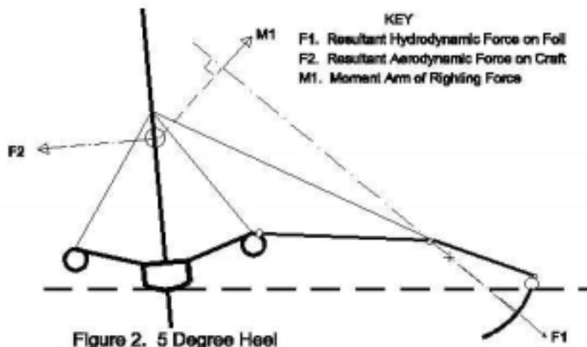
the craft is heeled 5 degrees to leeward of the dynamic equilibrium position. This small angle of heel creates a powerful righting moment due to the moment arm (M1). This tends to rotate the craft until it is upright when M1 will be zero. This is true for all wind strengths, and also if the craft heels to windward. The change in angle of F1 per degree of heel of the craft is the **Hapa Angular Gain**.
