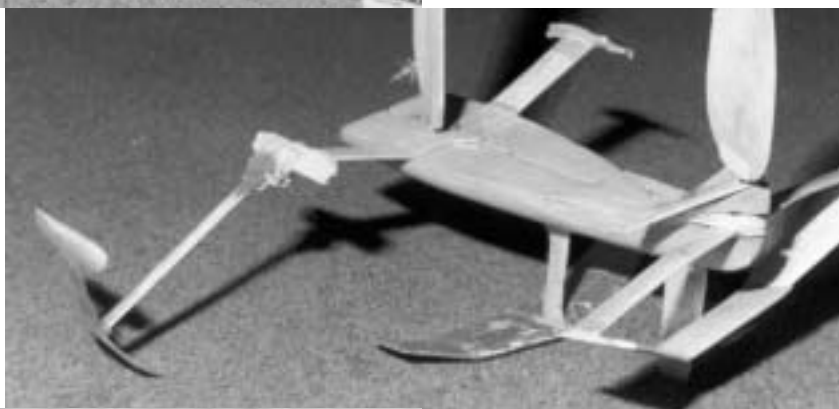
Figure 5. The 12" skiff was the first HSSC to plane on a reach, and achieve stable foilborne operation.
