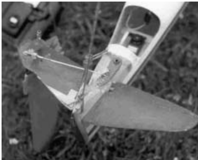
Figure 9. HS48 canard rudder showing servo linkage, arranged so that the rudder angle is unaffected when the rudder knocks up.
