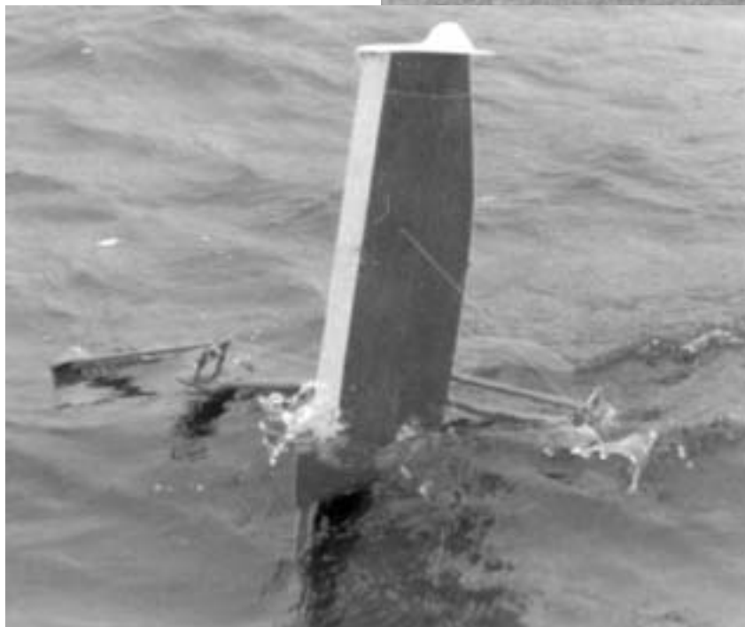
Figure 6. This 20" version was disappointing. In getting it to work, I fitted a vane steered canard rudder, moved the rig forward and raised it, lengthened the hull to 24" to cure the dragging transom, and doubled the effective span over the foils.
