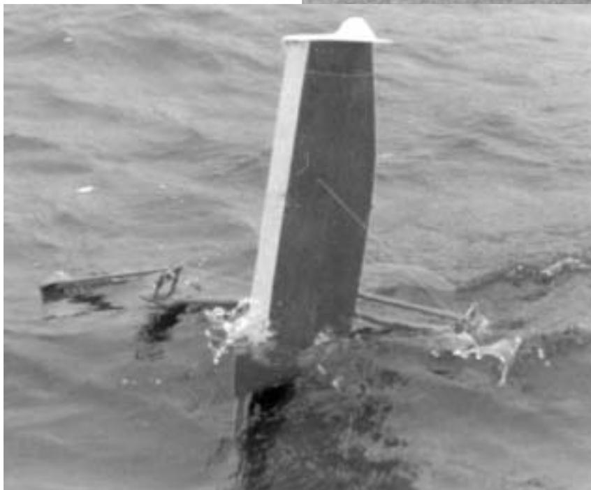
*Figure 6. This 20" version was disappointing. In getting it to work, I fitted a vane steered canard rudder, moved the rig forward and raised it, lengthened the hull to 24" to cure the dragging transom, and doubled the effective span over the foils.*
