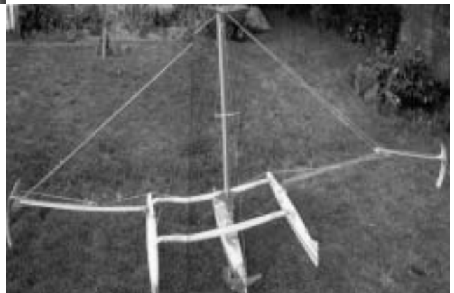
Figure 10. HS48 trimaran set up for port tack, rudder folded back, viking prows, swing wing akas, and self tacking wing sail (under-sized).
