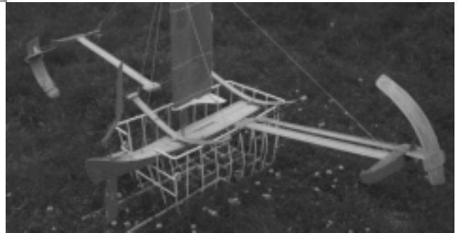
Figure 8. HS24 Skiff, with hapa deployed for starboard tack. These hapa foils are housed in daggerboard style cases, and are interchangeable rather than being handed pairs, so that only one type of foil is needed.
