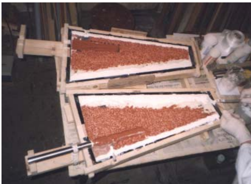
Figure 6 - Foil shell halves filled with "baked beans" prior to joining
