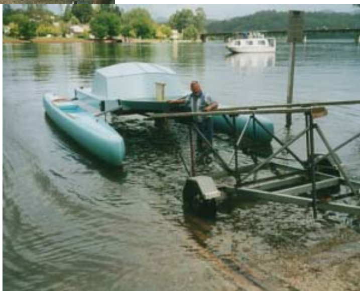
Photo 7 (below) - hulls spread to its sailing beam of 3.8m and the ends of the swing arms are bolted to the bridgedeck fittings
