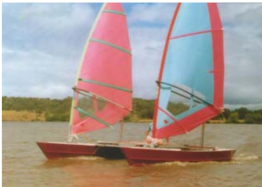
Photo 1 - Windrigger 5600 powered by 2 sailboard sails of 7 sqm each.
