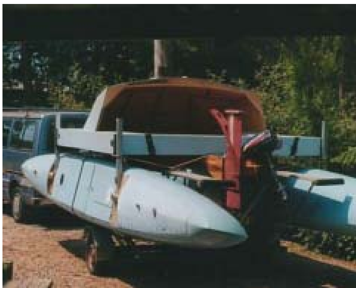
Photo 5 (above) - the cat is carried on its trailer with the hulls folded under its bridgedeck so that its beam 2.5m, the legal maximum towing width.
